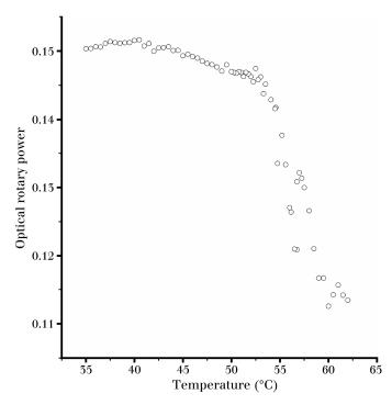
Figure 5. Variation of ORP (deg  $\mu m^{\text{--}1}\!)$  with temperature in the SmC\* phase
