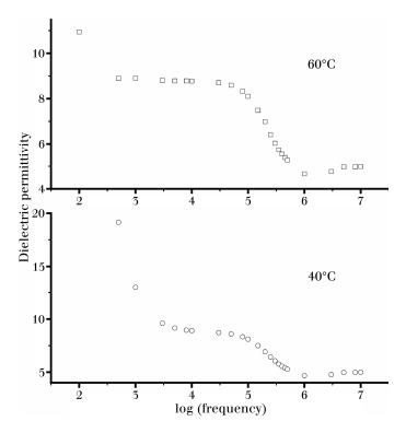
Figure 1. Variations in dielectric permittivity with the log of frequency (Hz) at 60°C and 40°C
