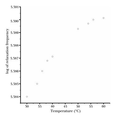
Figure 4. Relaxation frequency (Hz;  $f_{\rm r})$  as a function of temperature
