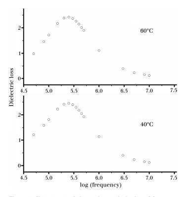
Figure 2. Variations in dielectric loss with the log of frequency (Hz) at 60°C and 40°C
